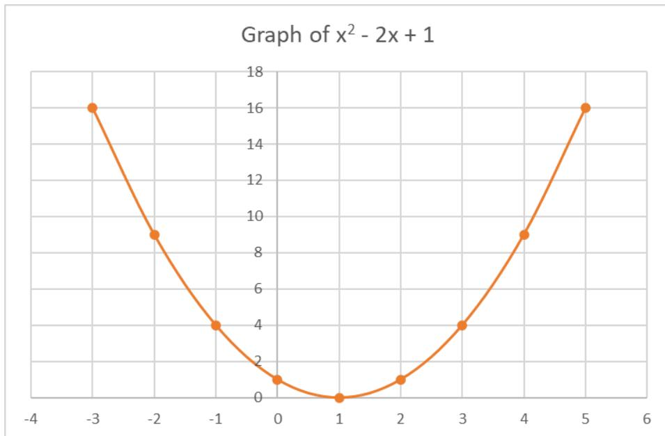
Notice our root (the point where the curve hits the x-axis) is at (1, 0). Notice the zero in the y coordinate slot. That's why we set the polynomial equal to zero and solve for our x coordinates. The x coordinates that we find are called the roots of our polynomial.
